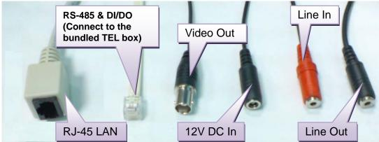
RJ45 LAN socket: Connect to PC or Hub/Switch. For connect to 10Base-T Ethernet or 100Base-TX Fast Ethernet cabling. This Ethernet port built N-Way protocol can detect or negotiate the transmission speed of the network automatically. Please use Category 5 "straight through" cable to connect the ICA-601 / ICA-651 to a 100Mbps Fast Ethernet network switch or hub.
